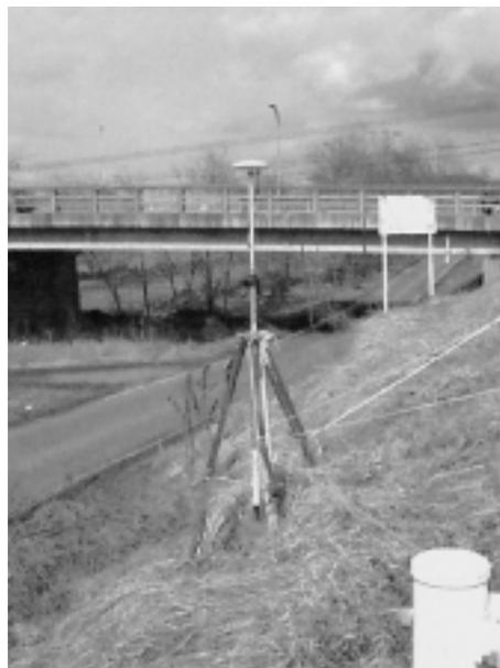
Fig. 2 An example of the antenna establishment conditions of the reference station.
