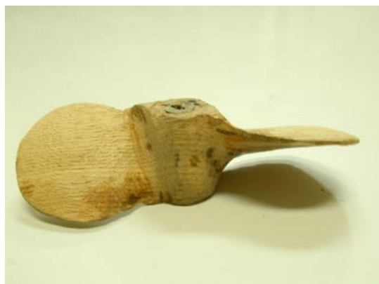
Photo.1 Model propeller made from wood
