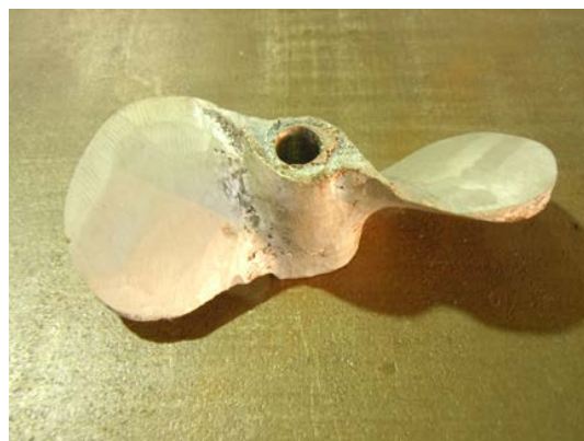
Photo.2 Molten model propeller
