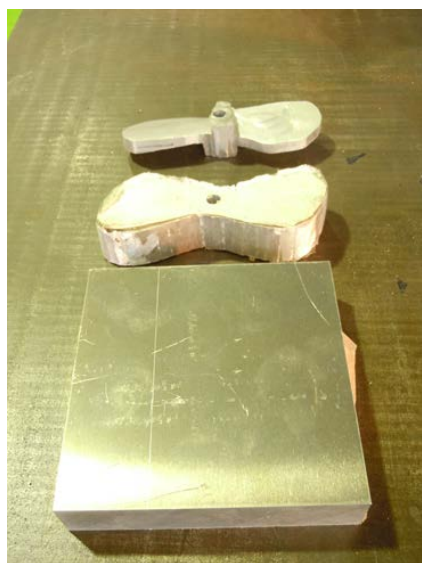
Photo.3 Model propeller of the manufacturing process
